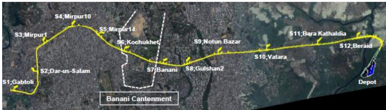
Alignment of MRT Line 5 corridor
